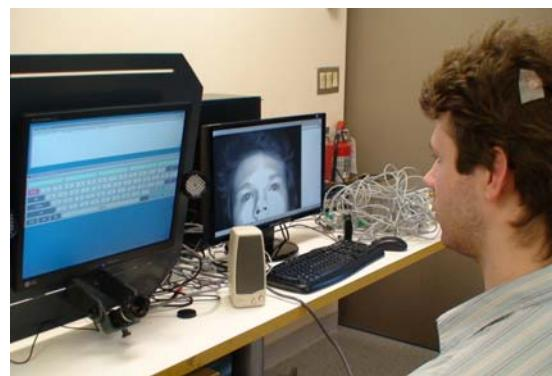
Fig. 2 – The participant controls the position of the cursor with his gaze and generates “click” commands by invoking motor imagery.
