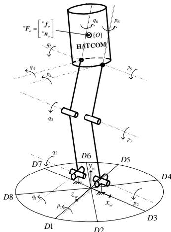
**Fig. 1:** Dynamic model of quiet standing with twelve DOF ( $q_i$  and  $p_j$ ) and eight perturbation directions (D1 to D8).
