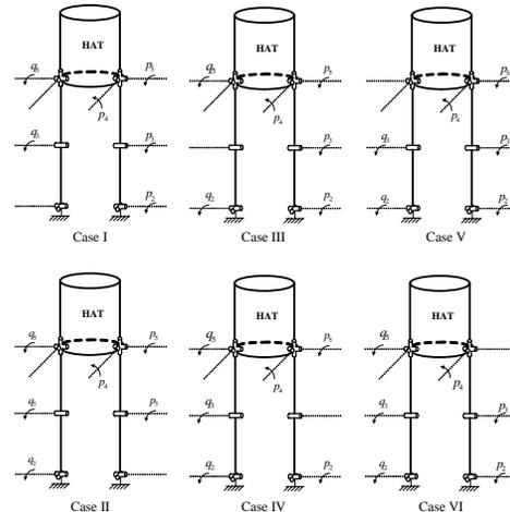
**Fig. 2:** Six cases of six DOF that need to be actuated in order to facilitate stable standing when external perturbations are present.
