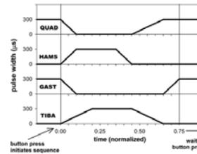
**Stimulation program for a single leg.** The stimulation begins from initial state representing late stance phase, and pushbutton triggers open-loop sequence beginning with swing phase (Thrasher et al. 2005).
