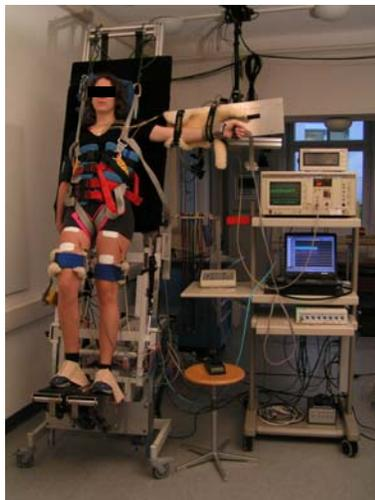
**Fig1** – Experimental setup. Subjects remained supine for 10 minutes, then were tilted 80° from horizontal for up to 30 minutes. BP, HR and EKG were recorded throughout all trials.
