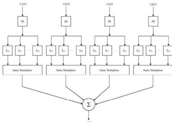
Fig. 2 – EMG-force model with inputs  $x_i(n)$  and output  $y(n)$
