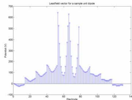
Fig2 – Influence of a unit current dipole on the electric potential at each electrode contact. The dipole corresponding to this vector is oriented in the x-direction and situated at the periphery of the endoneurium, halfway up the cuff electrode.
