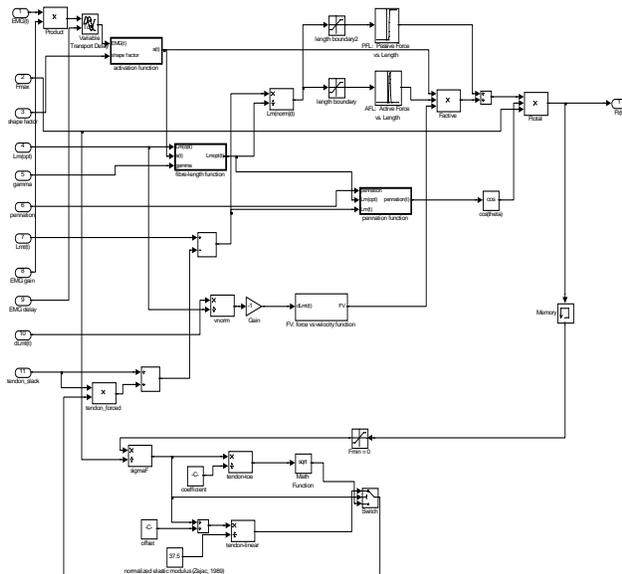
Fig1 – muscle model in simulink
