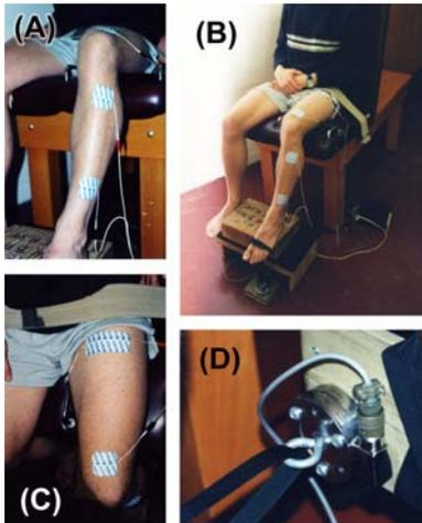
**Figure 1** – Electrode placement on the (A) tibialis anterior and (C) quadriceps. (B) shows the upright sitting position of each subject and (D) shows the uniaxial, strain gauge-based load cell used to measure force (Honeywell Sensotec, Columbus, Ohio, USA).
