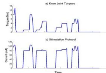
Fig. 3. a) Knee joint torque that facilitate “down hill” walking, b) Stimulation protocol applied to hamstrings m. that generates desired knee torque in a).
