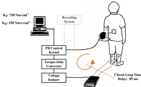
Fig. 2: Schematic Diagram of the Experimental Setup.
