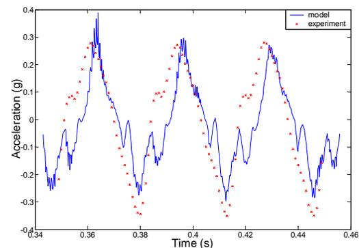
Fig. 2 – Acceleration of Femur, Model and Experimental Results
