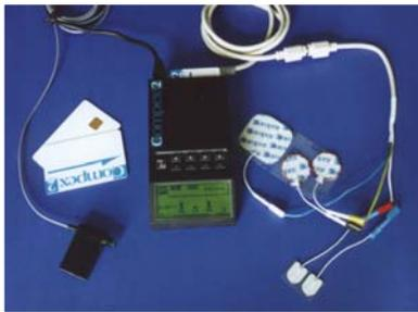
Fig. 1: Complex Motion Stimulator with surface electrodes (Compex SA, Switzerland)
