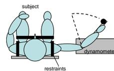
Fig2 – experimental setup (top view)
