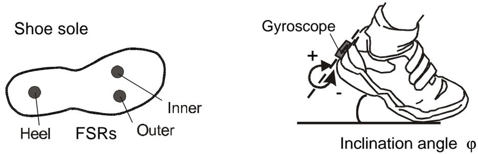
Figure 1: Placement of the sensors used by the Gait Phase Detection System.
