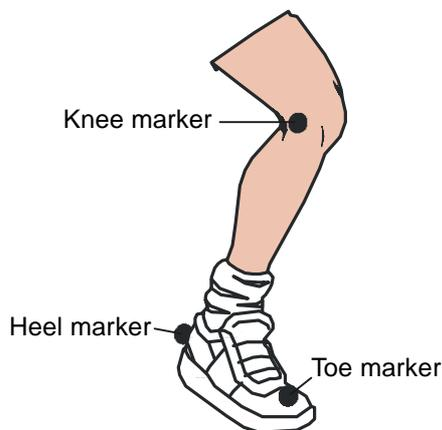
Figure 3: Positions of the retroreflective markers that were placed on the knee, heel, and toe. The Vicon measurement system tracked and measured the three-dimensional trajectories of these markers during the experiments.
