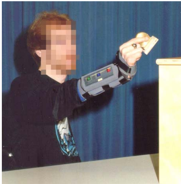
Figure 4: Bionic Glove developed by Prof. Arthur Prochazka from the Univesrity of Alberta, Canada (courtesy of Prof. Arthur Prochazka)
