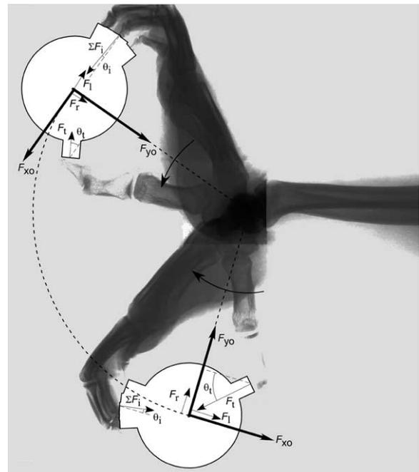
Fig. 3. Schematic representation of the force vector equilibrium during the isokinematic phase of active wrist motion against load with  $\sum_{i=1}^4 F_i + F_t + F_l + F_r = 0$ . ( $\sum_{i=1}^4 F_i$ : sum of the individual finger forces,  $F_t$ : thumb force,  $F_l$ : applied load,  $F_r$ : reaction force to equilibrate the shift perpendicular to the wrist rotation axis.)
