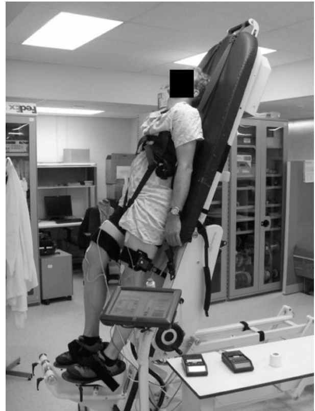
Fig. 1. The experimental setup. Subjects were secured onto the tilt-stepper with torso and shoulder harnesses. Actuators attached to the thighs perform passive movements. FES was applied to the left and right quadriceps, hamstring and gastrocnemius muscles.
