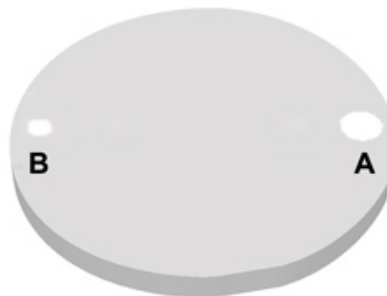
Figure 2. Illustration of galvanotaxis chamber. Strips of vacuum grease are used to create a pool of culture media on either side of the central trough.
